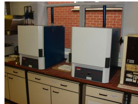
Kilns Loss on Ignition
